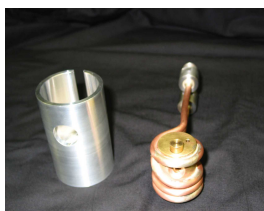
Circulating bath heated cell (up to 200°C) for powder samples in capillaries Backscattering geometry
